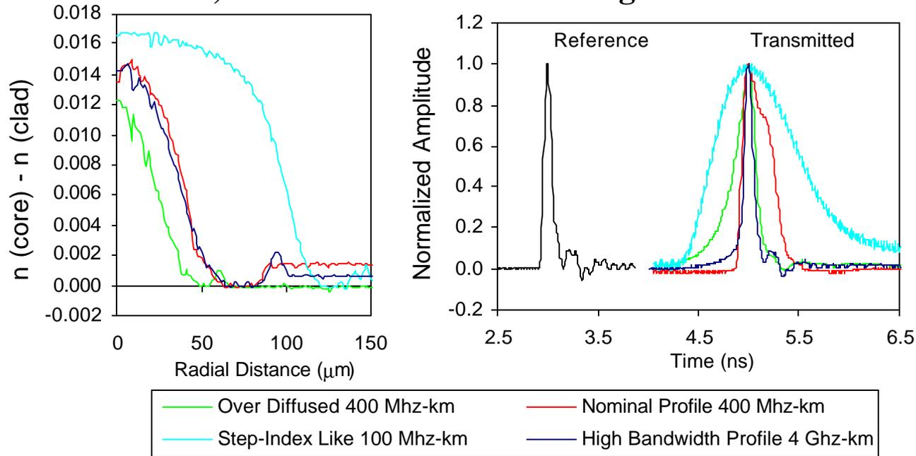
Differential Mode Delay measurements
