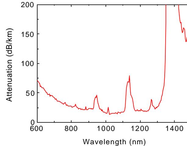
**Attenuation typically 25-35 dB/km at 850 nm**
