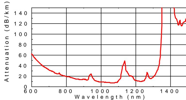
10-fold lower attenuation than PMMA-based POF
